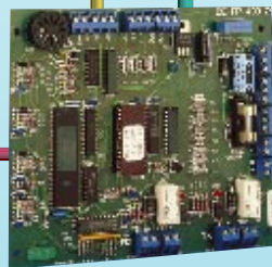
FM 808 Open collector output board 8 zones FM 816 Open collector output board 16 zones FM 832 Open collector output board 32 zones FM 864 Open collector output board 64 zones
