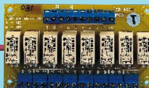
RB 808 8-way relay board for use with FM 800
